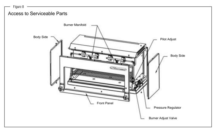
If necessary (or convenient), wall-mounted and flue-riser-mounted models can be un-mounted for servicing or repairs. Use two people since the Cheese Melter weighs about 175 pounds (79 kilograms). Refer to the installation procedure in the previous section of this manual for guidance.
